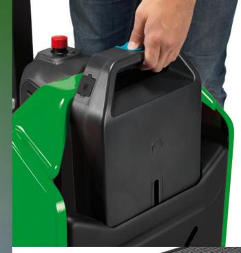
P013i: the powerful battery comes in cassette format, fully sealed and easy to handle. The connectors are protected so no risk of short circuits
